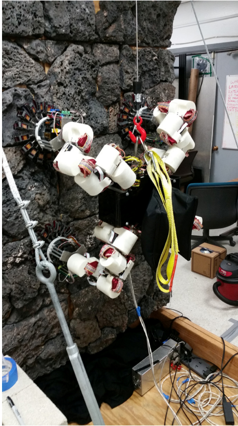
Figure 1: Prototype of the LEMUR robot under development at the Jet Propulsion Laboratory Rock Wall Test Facility. A version of this robot was recently tested in lavatubes at El Malpais National Monument, in Grants, New Mexico. LEMUR possesses unique footpads fitted with Microspines™ that grip rock using a series of circular arrays of sharp hooks, thus enabling secure clinging across a wide span of relative surface roughness conditions. The project goal is to integrate a variety of scientific instruments with such robots for access to lavatubes on Earth that may be inaccessible due to size, thermal characteristics, or gases poisonous to human investigators and to develop such capabilities for application to extraterrestrial mission targets including Mars and lunar lavatubes, and possibly cryogenic volcanic cavities on icy Solar System bodies. Image courtesy of A. Parness, NASA-JPL.
